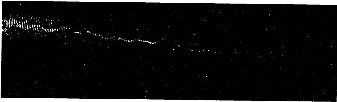
Figure 1.4 shows electron flow through the 1st mode ( G = 2e^2/h ) of a QPC. The electron flow is constrained to a surprisingly narrow branch throughout the entire scan range, and coherent fringes decorate the flow out to the edge of the scan. The QPC gates and channel are located approximately 300nm to the left of this scan.
