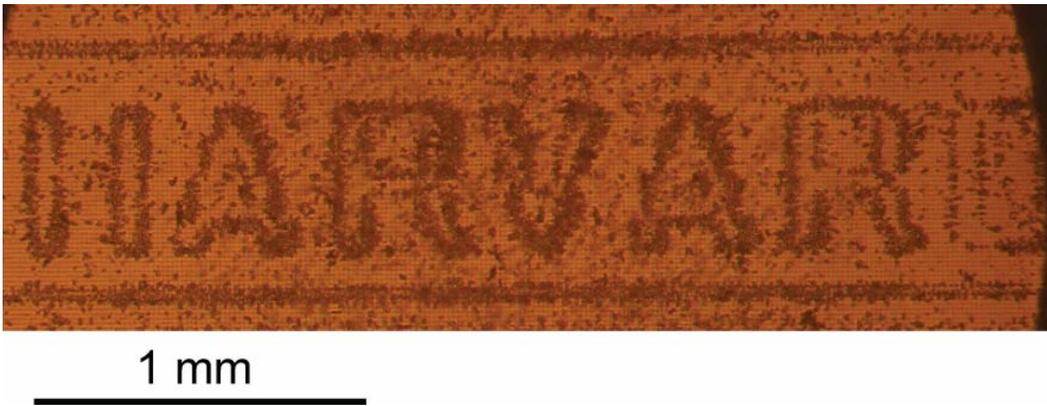
Figure 7.3 Complex pattern of thousands of yeast cells patterned by DEP. Pixels across the array were energized to spell out “HARVARD”, attracting cells toward the local maximum of the electric field.
