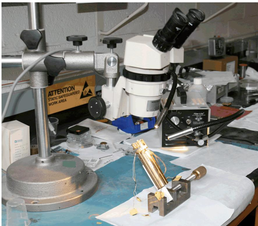
**Figure 3.8:** Setup to perform fine positioning of the tip over the device of interest. By viewing the tip and the sample on an angle, the tip's reflection is easier to see as the tip approaches the sample. A clear view of the tip's reflection makes it easier to tell when the tip is near the sample and to more accurately discern the lateral position of the tip over the number grid.
