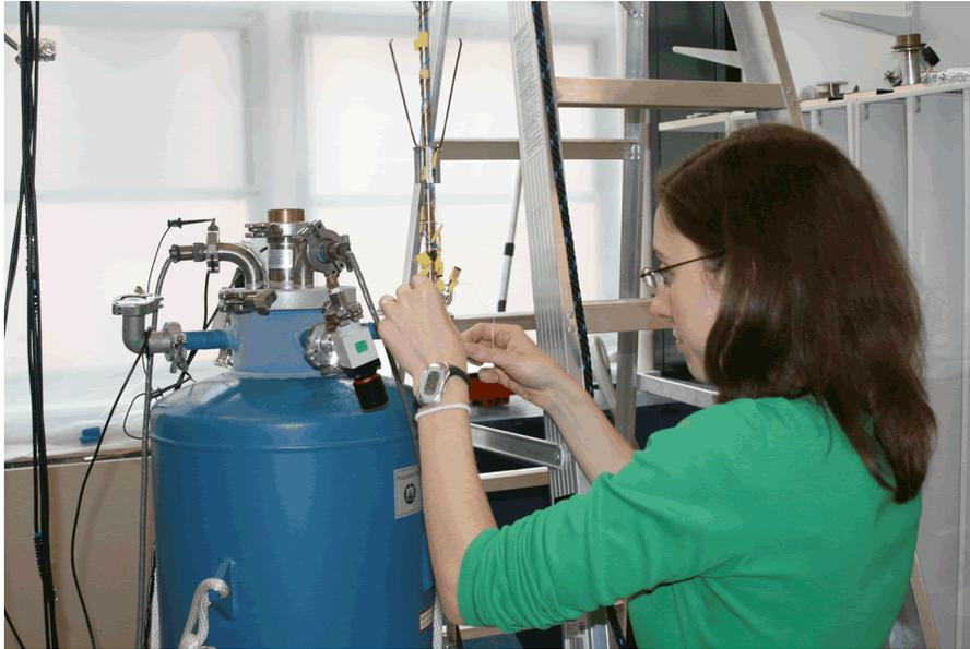
**Figure 1.4:** Preparing the SGM to cool down to liquid-He temperatures. (See chapter 3 for a detailed description of the experimental apparatus.)
